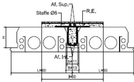
In the areas where brackets are more packed, place brackets of 6mm diameter as indicated in the drawing.
